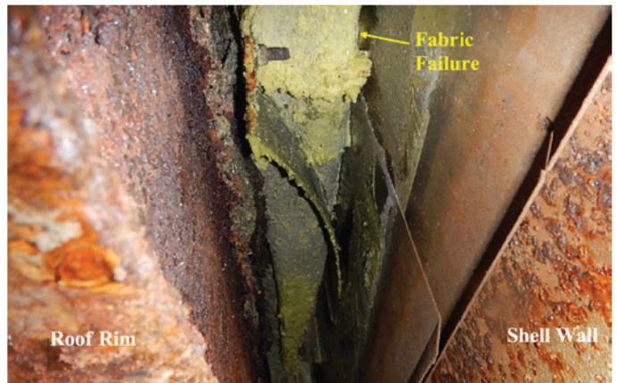
Figure 2. Hydrogen Sulfide ( H_2S ) buildup on chemically inert Teflon emissions control fabric with fiberglass scrim.
